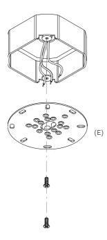
Note: Make sure the supplied Universal Mounting Plate is fastened directly to the junction box. The surface of the junction box should be set back 1/8" or 3mm from the mounting surface. This will ensure the best possible fit for ease of installation and final finish. Note below the correct and incorrect fit for optimum installation.
